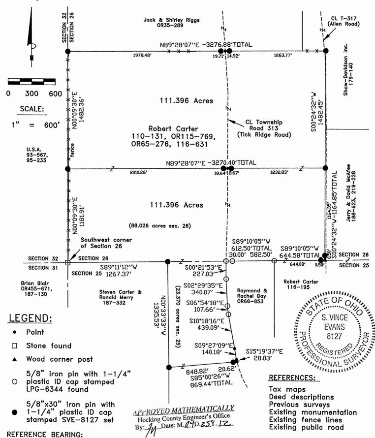
The west line of Section 26 as North 00 degrees 09 minutes 30 seconds East. Bearings are based upon an assumed meridian and are to denote angles only.
