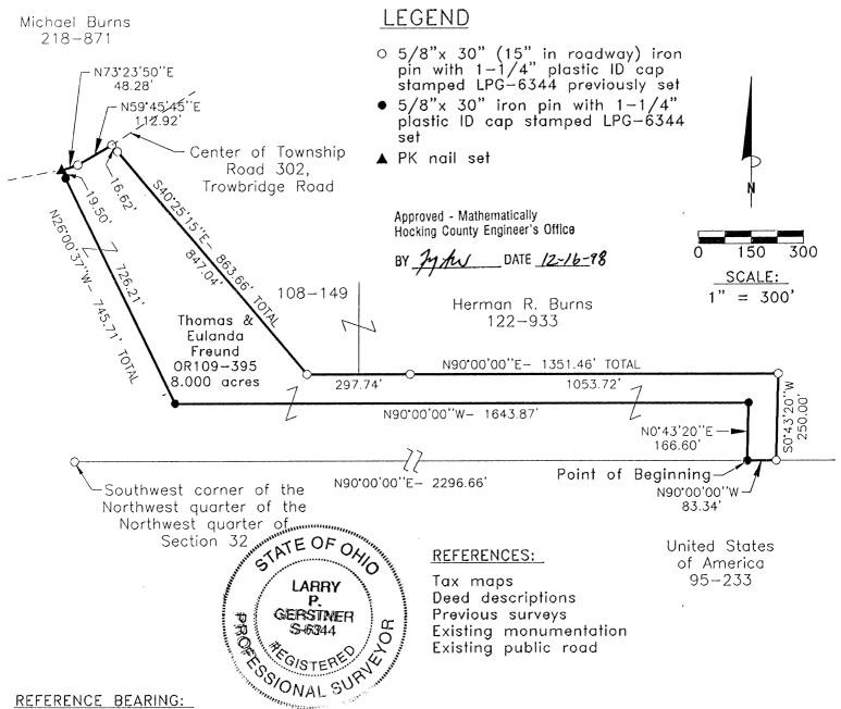
The North line of Section 32 as North 90 degrees 00 minutes 00 seconds East. Bearings are based upon an assumed meridian and are to denote angles only.
