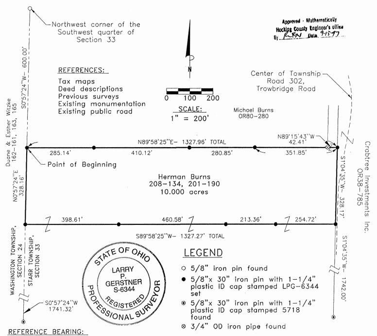
The South line of Section 33 as North 90 degrees 00 minutes 00 seconds West. Bearings are based upon an assumed meridian and are to denote angles only.
