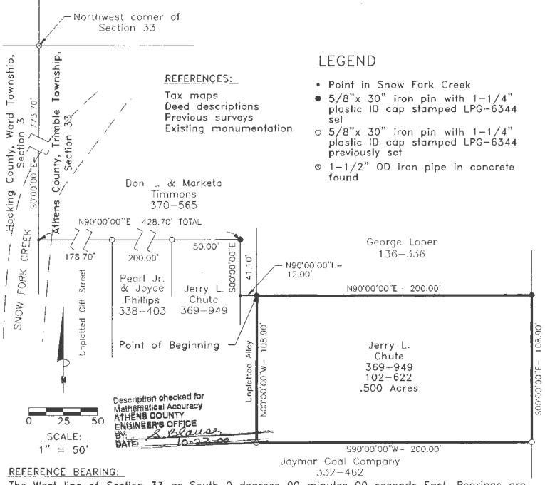
The West line of Section 33 as South 0 degrees 00 minutes 00 seconds East. Bearings are based upon an assumed meridian and are to denote angles only.
