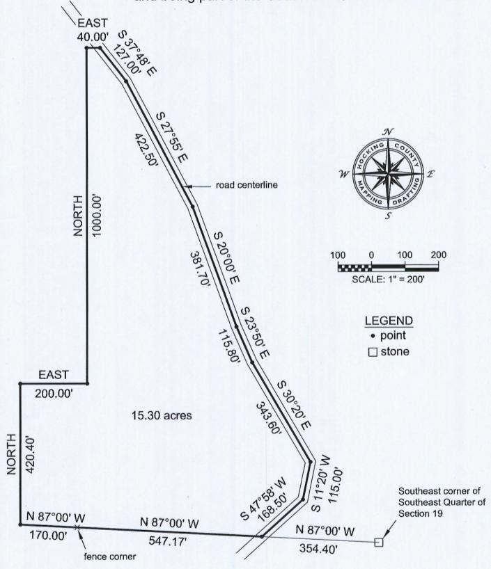
Note: This drawing is not a survey; it was created by the Hocking County Mapping & Drafting Department using the legal description on a deed to the State of Ohio, recorded in Deed Record Volume 100 at Page 481, Hocking County Recorder's Office.
