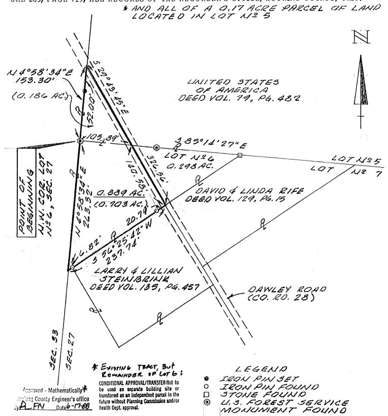
The bearing system for this plat is based on the east line of Section 34, Township 13, Range 15 as shown on a Plat of Survey by William M. Watkins dated October 6, 1984 on file at the Office of the Hocking County Engineer, Logan, Ohio.
