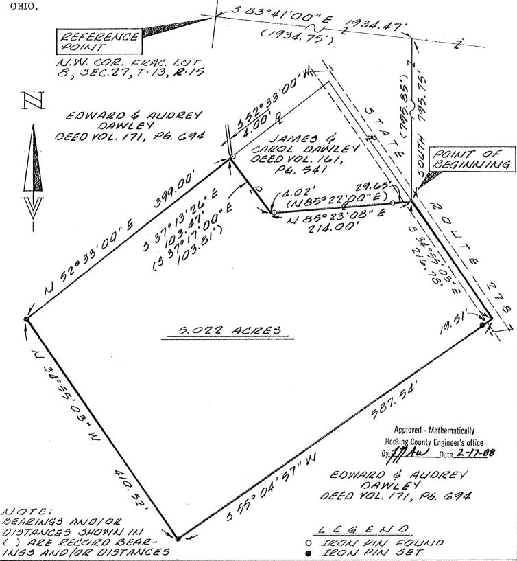
The bearing system for this plat is based on the north line of FRACTIONAL LOTS of Section 27, Township 13, Range 15 as being S 83° 41' 00" E.
