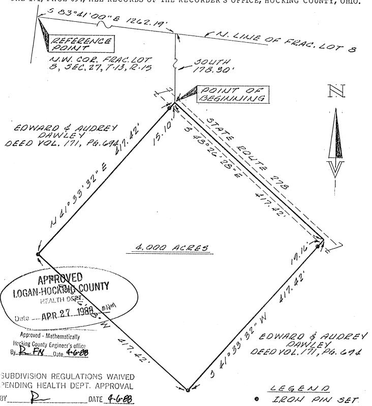
The bearing system for this plat is based on the north line of Fractional Lot No. 8, Section 27, Township 13, Range 15 as being S 83° 41' 00" E.
