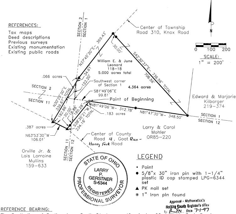
The South line of Section 1 as South 81 degrees 49 minutes 06 seconds East. Bearings are based upon an assumed meridian and are to denote angles only.
