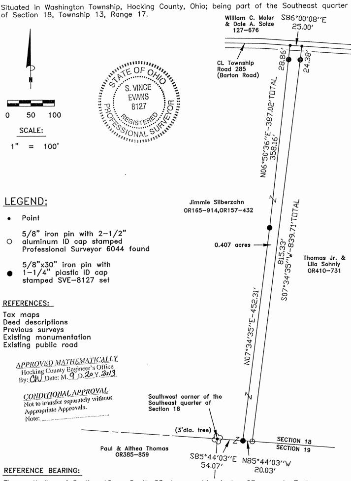
The south line of Section 18 as South 85 degrees 44 minutes 03 seconds East. Bearings are based upon an assumed meridian and are to denote angles only.
