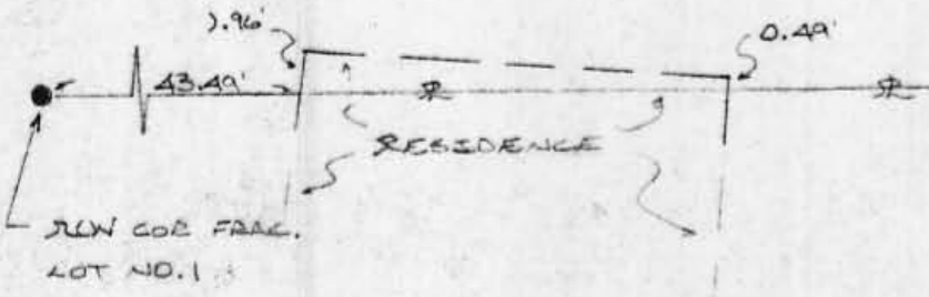
— DETAIL OF ENCROACHMENT — 1" = 10'
