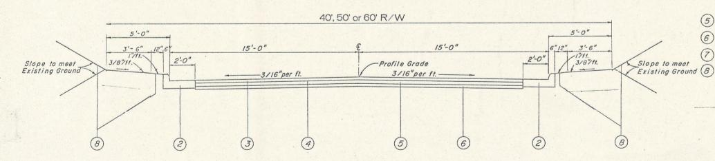
Type 2-A Monolithic Curb as per Plan (2) Combination Curb and Gutter (Ohio Department of Highways Std. Drawing 1-12, Type 2)
